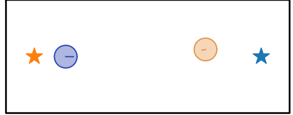
Figure 2: Two variants of the sidewalk problem. The goal is for each agent to navigate to its respective goal without colliding with the walls or other agent. Left: Discrete Domain. Right: Continuous Domain. The agents are modeled as unicycles, goals are depicted as stars.
